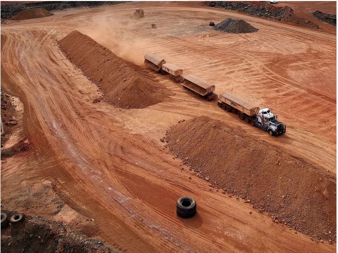
Unloading ore at the Davyhurst ROM pad
