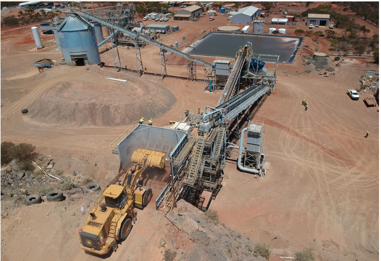
Loading commissioning ore into crusher at Davyhurst Process Plant
